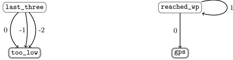
(a) An annotated dependency graph for the stream last_three . A monitor for last_three needs to save the last two events of too_low .
